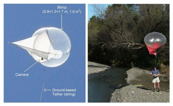
Figure 1. The SkyHook helikite. A 1.6 m<sup>3</sup> combined blimp-kite, with simple pan-tilt camera mount, secured by a ground-based tether. The blimp-kite is operated by a single person on the ground using a reel to control the height of the kite and walking to control its position. This figure is available in colour online at www.interscience.wiley.com/journal/rra
