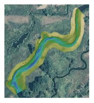
As compared with the regular DEM, this detrended DEM does a nice job of highlighting the pools, bars and floodplain.
