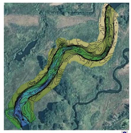
3. If you wish to check the elevation of a particular contour use the *Identify tool* to see its elevation. If you want to label the contours, right click on the contour layer and in the Properties Dialog go to the Labels tab and adjust the settings.
